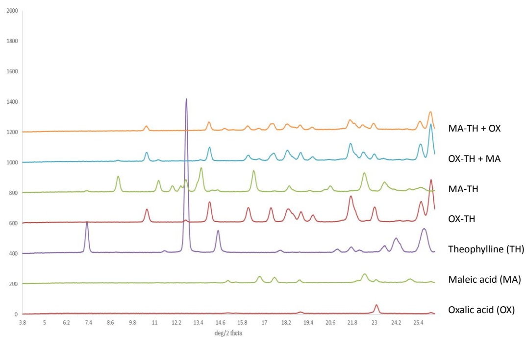
Figure 2.7. PXRD patterns obtained for the CCF exchange reactions of OX-TH and MA-TH.
